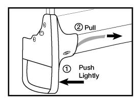
(10) Push lightly forward on the bottom of the splash guard. Slowly pull the tape backing tab rearward to remove.
