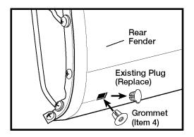
The procedure below shows the installation for the left side. Repeat the same procedure for the right side.
