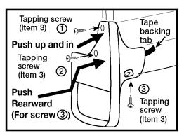
The procedure below shows the installation for the left side. For the right side, use standard bed instructions.
