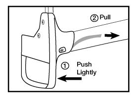
(11) Push lightly forward on the bottom of the splash guard. Slowly pull the tape backing tab rearward to remove.
