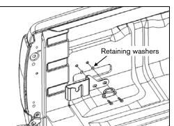
1) Remove the bolts that secure the tiedown hooks with a 12 mm wrench. **Do not** discard bolt and tiedown hooks.
