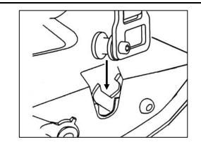
When the Bed Extender is at the furthest rear position, push down on the buckle to insert into tailgate latch. Tighten straps. To release, pull tailgate handle.
