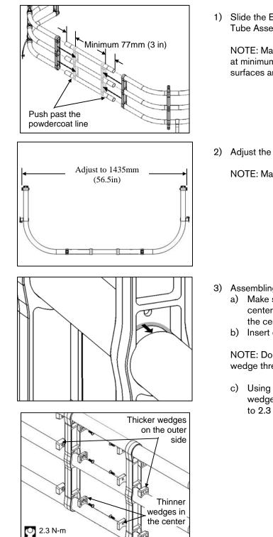
I) Slide the Extension Tubes evenly into the Left and Right Bent Tube Assembly.
