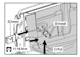
(Truck without drop-in bedliner, skip this step). Pull the bedliner away from the truck bed sheet metal to insert the Bolt-On Brackets. Re-install the Tie Down Hooks as shown in figure. Tighten the bolts that were removed in previous step to 11-16 N-m (97-142 in-lbf.).
