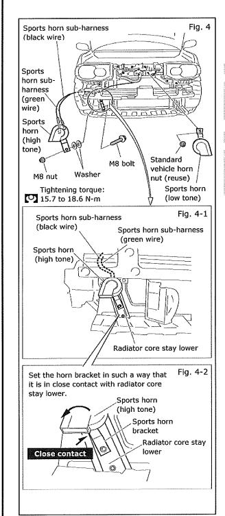
e) Align the sports horn and install the fasteners as shown.
