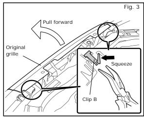
d) Using needle nose pliers, squeeze clips B on the back side of the original grille and pull forward on the top portion of the original grille to disengage the clips B from the vehicle. See Fig. 3.
