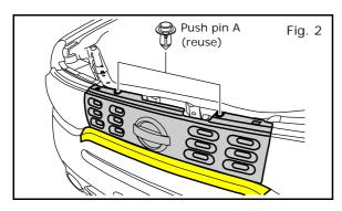
c) Use a clip remover to remove push pins A(reuse). See Fig. 2.
