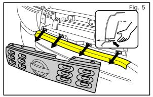
f) By hand, unhook the original grille claws from the front bumper and slowly remove the grille by pulling the grille away from front bumper. See Fig 5.
