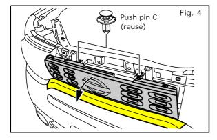
e) Use a clip remover to remove push pins C(reuse). See Fig. 4.
