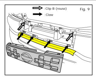
c) Align the Extreme custom grille clips B and claws to the holes in the front bumper and push the Extreme custom grille against the front bumper to insert the clips B and claws in the holes. See Fig. 9.
