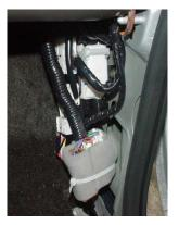
Without AMP: Secure to lower bracket opening.
