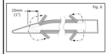
8) Peel back tape liner 25 mm (1") from all 4 ends, as shown in Fig. 6.
