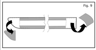
12) Remove tape liner from both ends of Rear Body Side Molding, as shown in Fig. 9.
