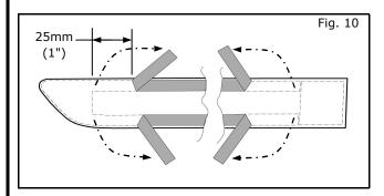
13) Peel back tape liner 25 mm (1") from all 4 ends, as shown in Fig. 10.
