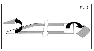
7) Remove tape liner from both ends of Front Body Side Molding, as shown in Fig. 5.
