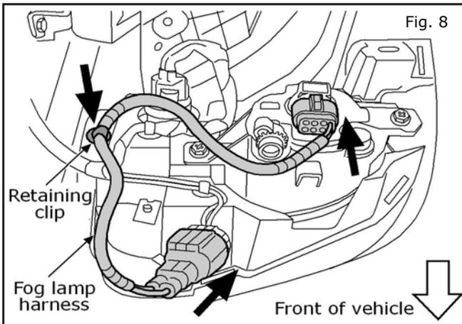
8. Plug the fog lamp harness into the connector at the back of the fog lamp. Plug the other end of the harness into the pre-wire vehicle harness connector.
