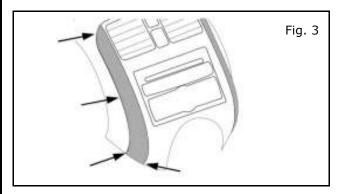
5) Carefully and lightly place part in upper corner first aligning cluster finisher with center edge grove.
