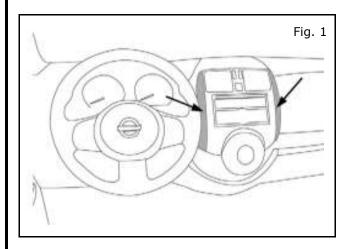
Use an alcohol wipe to clean the indicated areas on the vehicle where the cluster finishers (LH and RH) are to adhere.
