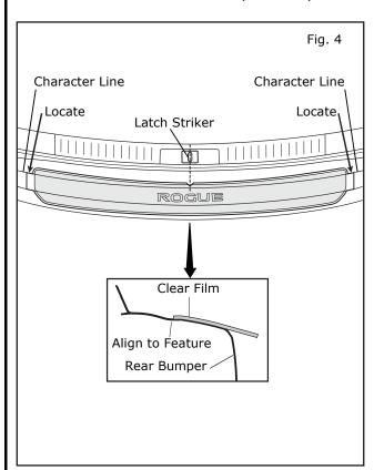
5) Align film into position with notch to latch striker and film locator to character line.
