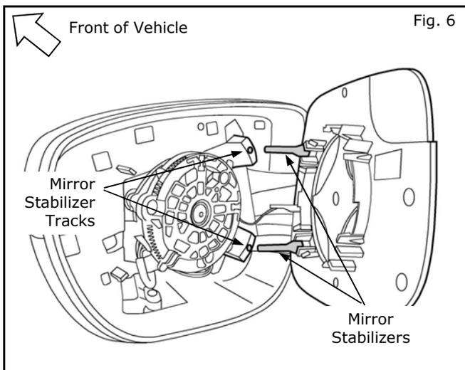
6) During installation, be sure that the two **mirror stabilizers** are lined up with the two stabilizing tracks in the mirror housing as the mirror assembly is placed into position over the glass actuator.
