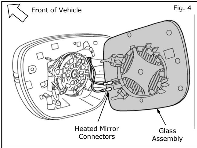
4) Carefully remove the glass assembly from the mirror housing.
