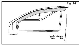
16) Replace rubber weather strip and make sure it is fully seated. Remove masking tape.
