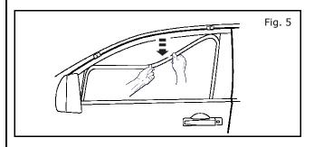
6) Set deflector aside and pull rubber weather strip down to expose door flange.
