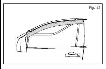
14) Remove tape liner by pulling on exposed pull tab.
