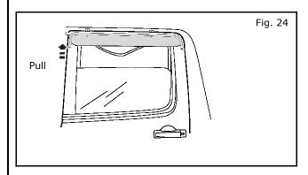
28) Remove front vertical tape liner and tack deflector in place.
