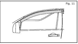
13) Remove rear tape liner and tack deflector down in place.
