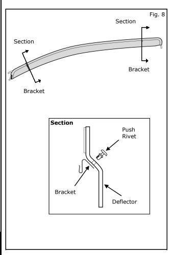
9) Attach brackets to deflector using push rivets.
