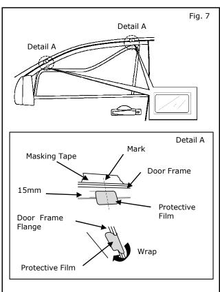
8) Place protective film 15mm from bottom edge of door frame centered on marks on masking tape and wrap to inside of door frame.
