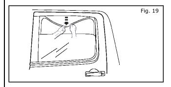
23) Set deflector aside and pull rubber weather strip down to expose door flange.
