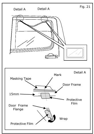
25) Place protective film 15mm from bottom edge of door frame centered on marks on masking tape and wrap to inside of door frame.
