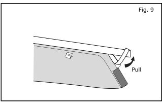
10) Pull and remove tape liner completely from front flange of deflector.
