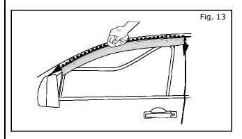
15) Using a clean cloth apply at least 15 lbs. of pressure along tape length.
