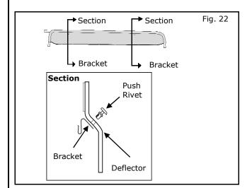
26) Attach brackets to deflector using push rivets.
