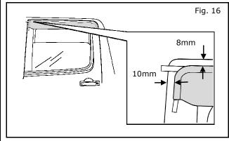
20) Ensure there is an 8mm gap between top flange of deflector and door edge and 10mm gap between front flange and front of door.
