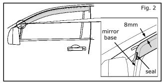
3) Place deflector so seal compresses against mirror base and deflector is 8mm below door edge.
