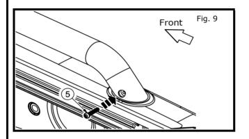
Assemble side rail tube to base using 8mm x 45mm long bolt. Tighten all bolts using 5mm allen head drive. Torque to 16 ft·lbs. Repeat for all corners.
