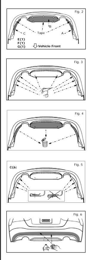
2) Apply masking tape to drilling templates A, B, and C at the locations indicated on template. Templates indicate edges with arrows that bump up to the edges on fascia.
