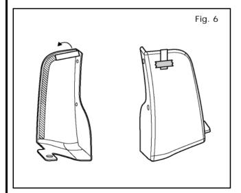
7) Fold tape liner pull tabs onto rear splash guard surface and apply masking tape to ensure that pull tabs are accessible.
