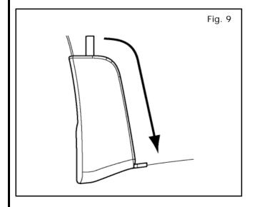
10) Remove tape liner in direction shown by arrow.
