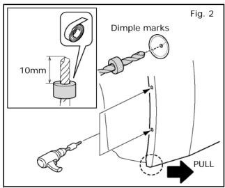
2) Pull out on bumper and Drill 3mm(1/8")→6mm(1/4") holes at 2 marked locations.
