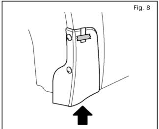
9) While pushing up splash guard from bottom, tighten phillips screws (E) as shown in Fig. 8.
