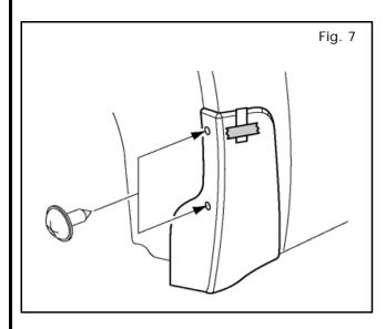
8) Align rear splash guard to vehicle and loosely install phillips screws (E).
