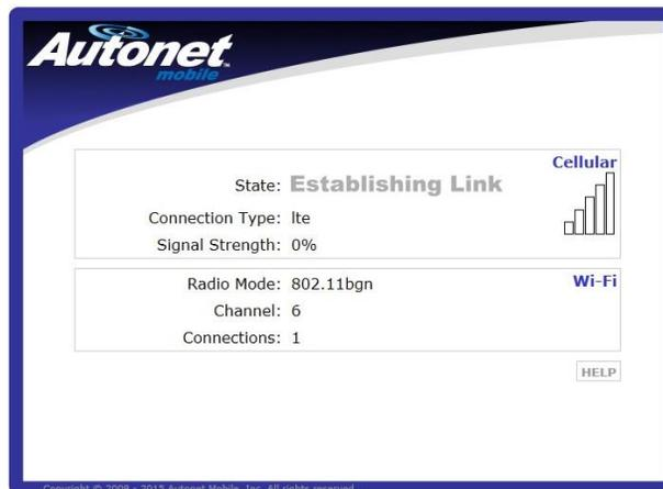
If you are unable to see the "Autonet-XXXX" in your wireless network list verify power is present to the WiFi module. If power is present and module still does not appear on the wireless network list call Autonet Mobile at 1-800-977-2107
