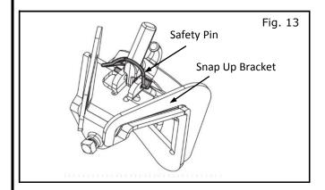
**NOTE: Secure Safety Pin to Snap Up Bracket**
