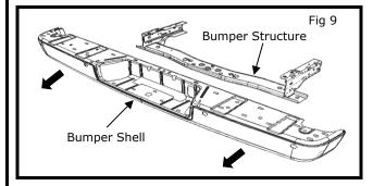
c) Slide bumper shell off of bumper structure. See Fig. 9 Bumper structure can be discarded.
