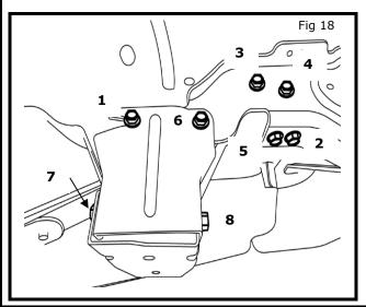
b) Torque all bolts to 133Nm in sequence shown.
