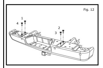
Loose install four M10 torx bolts into top of Bumper/Hitch assembly. Following the torque sequence in Fig. 12, torque bolts to 35 +/- 5 Nm
