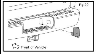
b) Install trailer tow 7/4-pin connector to bumper as shown.
