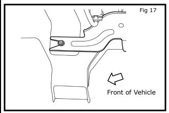
Ensure hitch assembly is engaged with forward bolt as shown in fig 17 on both sides of vehicle)
