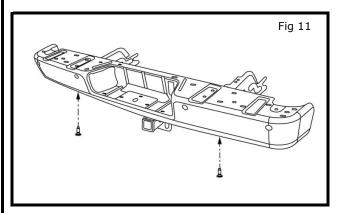
b) Install two M10 torx bolts into bottom of Bumper/Hitch assembly. Using T-45 torx socket torque bolts to 35 +/- 5 Nm. See Fig. 11.
