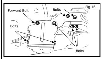
a) Align Bumper/Hitch Assembly and plate to Frame mounting holes. Loose install eight(8) bolts on inside of vehicle frame(8Rh/8Lh). See Fig. 16.
