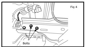
Remove two rearmost attachment bolts(2 Rh/2 Lh) using 17mm socket. See Fig. 3. Discard M12 bolts.
