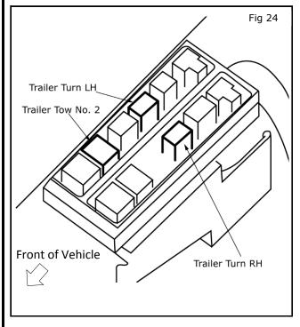
b) Install the two Turn Signal Relays (25230-79917) and one Tow Relay (25230-7996A) into the main fuse box. See fig. 22
