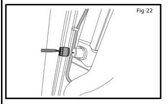
d) Connect jumper harness to 7/4 pin connector.
