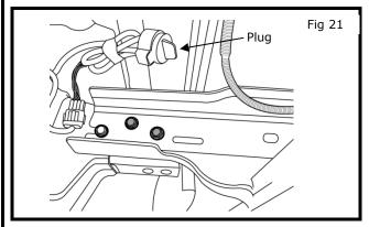
c) Remove protective plug from vehicle side harness
